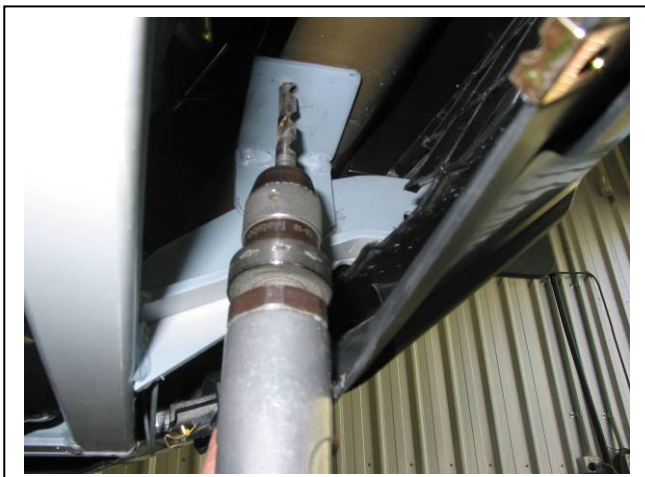
Figure 17 – Shown drilling cross member on passenger side
