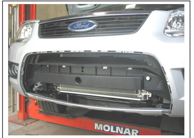
Figure 4 – Bumper with grille section removed.
