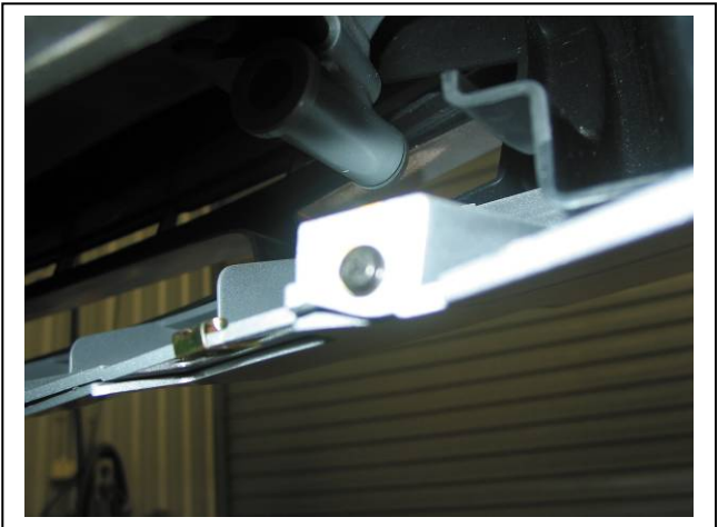
Figure 3 – PK screws on lower rear on bumper
